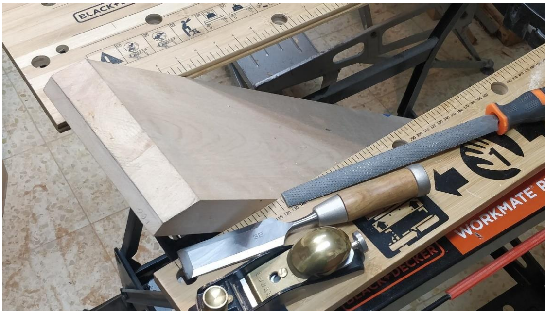
Shaping the bevel at the top of the chop
