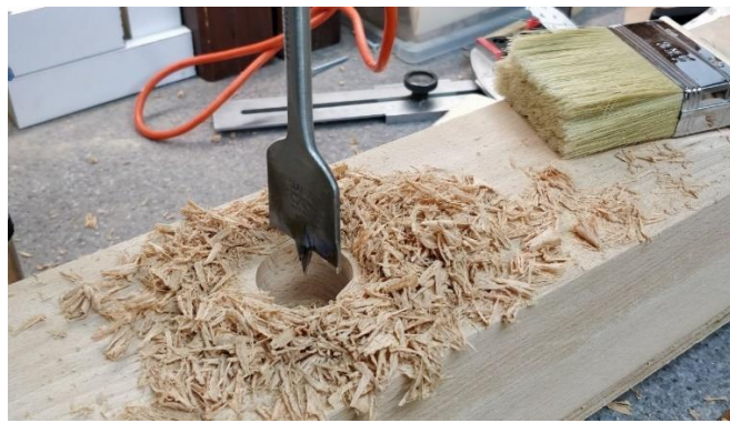
Drilling the hole for the vise screw
