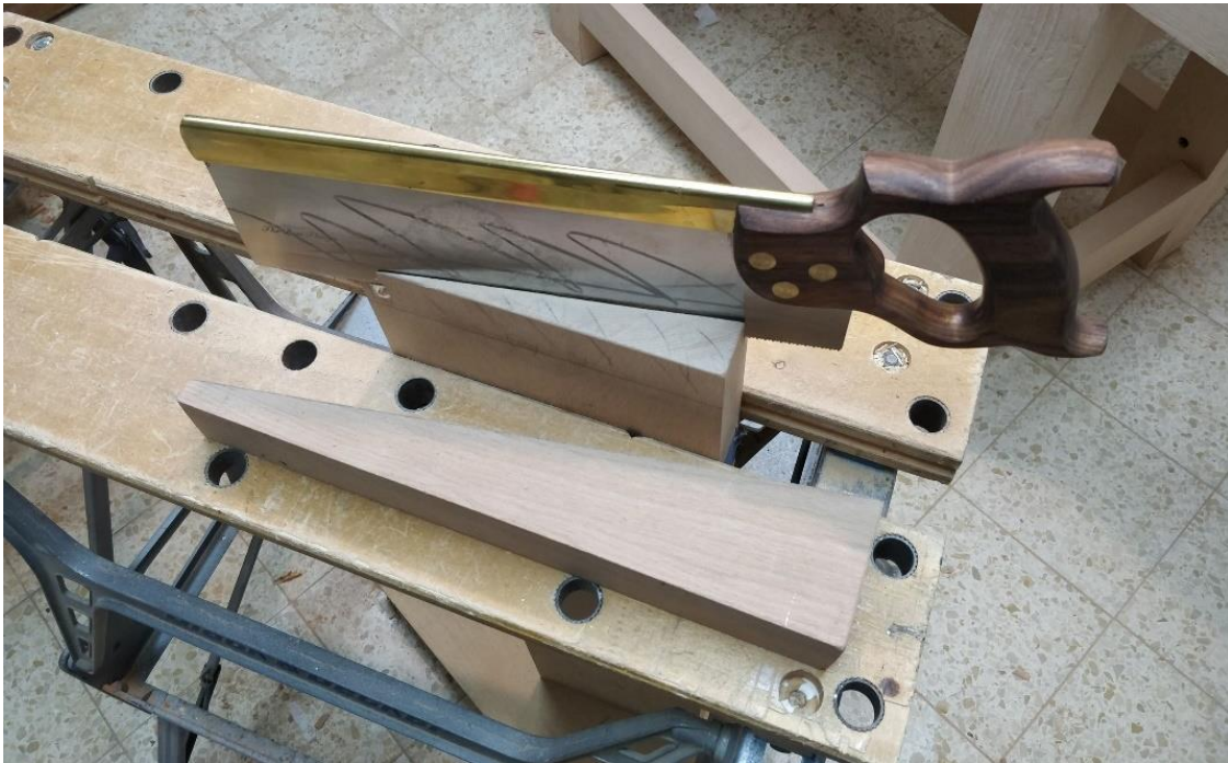
Cutting the rabbet for the spacer wedge
