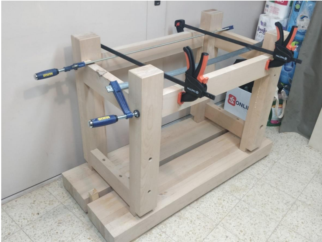
Gluing the long stretchers to complete the base
