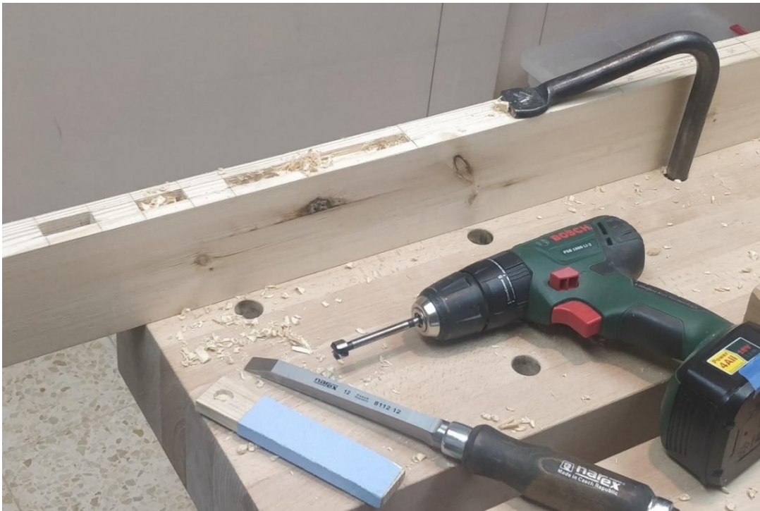
Cutting the slots in the gap stop
