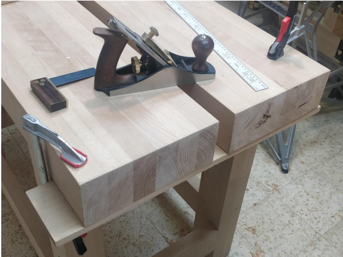
End planing setup – note the backer board below
