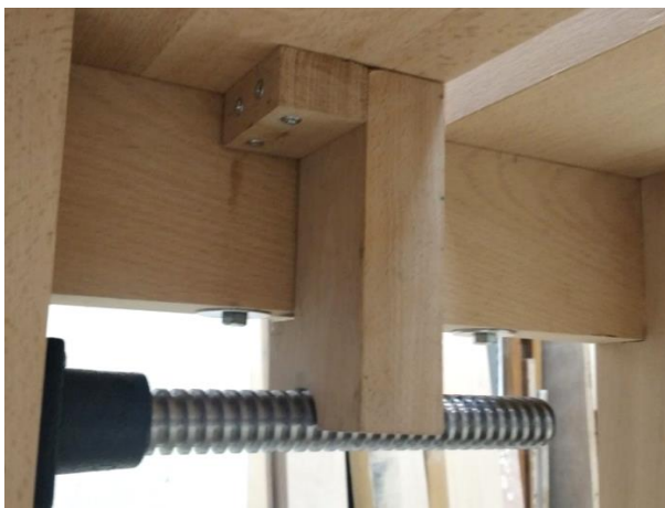
Spacer to keep the screw horizontal
