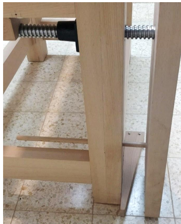
Right: Vise chop stabilizing solutions – Spacer above screw, dowel through leg, and wedge on the floor
