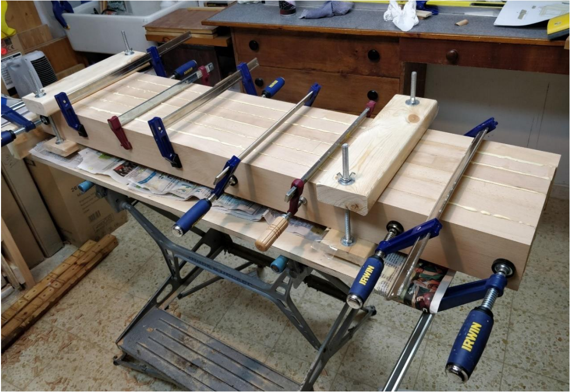
A benchtop slab being glued in the jig
