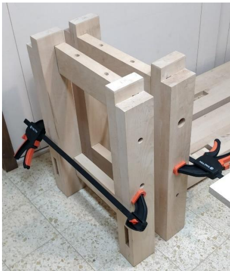
Dry testing the base end sections
