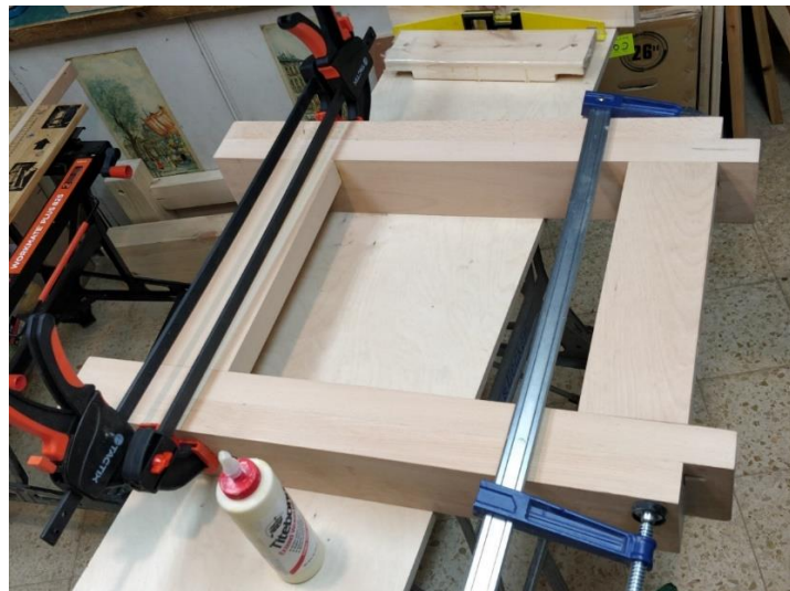
Gluing up an end section of the base
