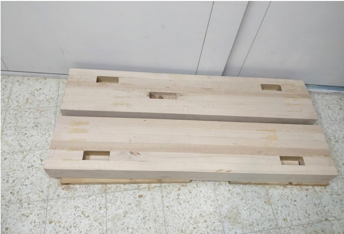
The two glued slabs, bottom side up. The “spare mortise” is where a defect in the wood was cut out; it will later be plugged with a matching piece of wood
