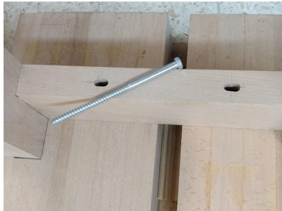
Elongated holes in an upper stretcher
