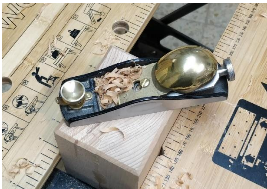
Chamfering the bottom of a leg
