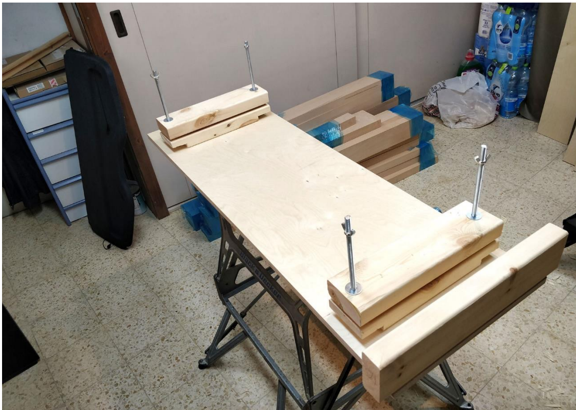
The lamination jig with its cauls and end stop
