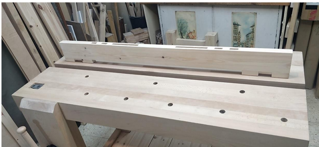
The finished gap stop, ready to go in its place
